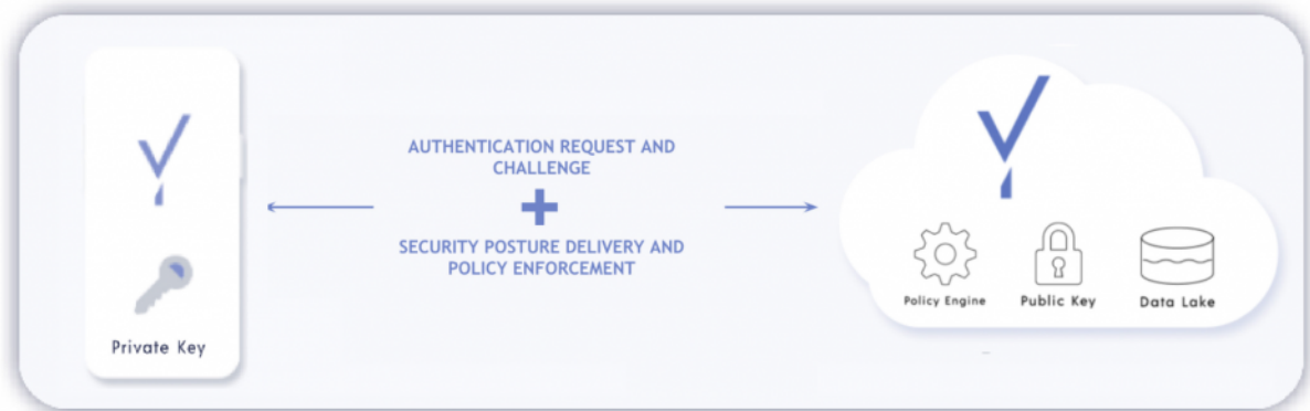
Figure 2: The authentication flow of Beyond Identity Secure Customers [Provided by Beyond Identity]
