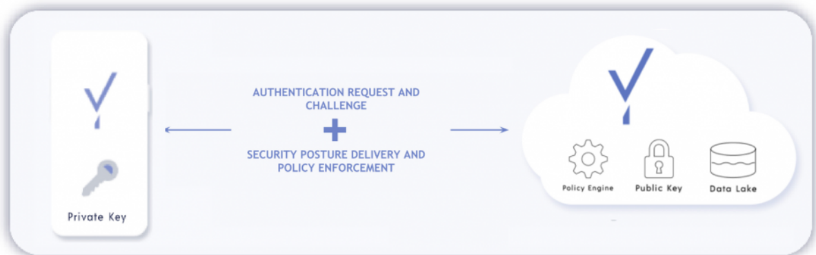
Figure 1: The authentication flow of Beyond Identity Secure Customers [Provided by Beyond Identity]
